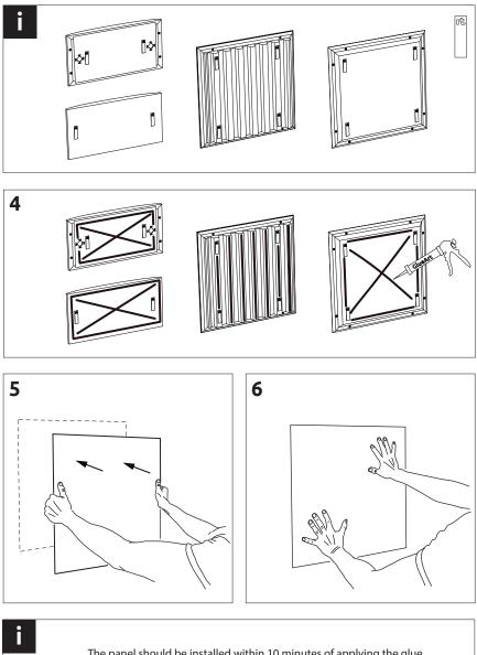
The panel should be installed within 10 minutes of applying the glue.
